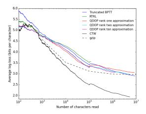
Compression rate (bits per characters) as a function of the number of characters read, for predicting the next character in Shakespeare's complete works.
