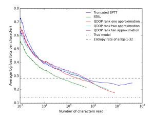
Compression rate (bits per characters) as a function of the number of characters read, for predicting the next character of  $a^n b^n$  sequences using a leaky RNN model.
